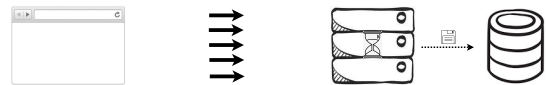
Figure 4: Running multiple concurrent user traces against the web application. An active query delay is active to force the exploitative interleaving needed to validate the GRC. The occurring sql log data is collected
